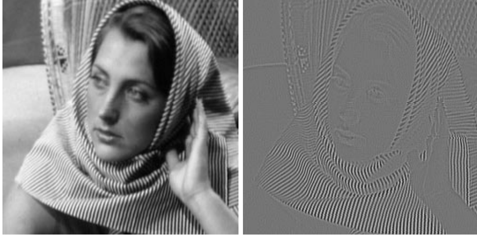
Figure 13: Projection onto V_{j_{max}} : real part (left) and imaginary part (right) of P_{V_{j_{max}}} I . (The original image is the right image displayed on Fig.19).
