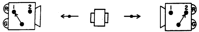
Fig. 1. The Hardy gedanken demonstration. Two particles emerge from a common source heading for two far apart detectors, each of which can operate in two modes, specified by the setting of a switch. When a particle reaches a detector the detector flashes a red or green light. Aside from the passage of the particles from the source to the detectors, there are no connections between the source and the detector or between the detectors.
