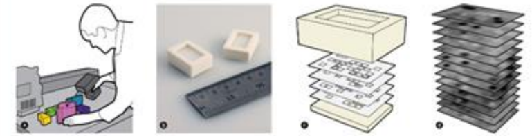
Figure 1: InfraStructs are material-based tags that embed information inside physical objects for imaging in the Terahertz region. Terahertz imaging can safely penetrate many common materials, opening up new possibilities for encoding hidden information inside digitally fabricated objects. (a) InfraStruct tags are embedded during the fabrication process to immediately identify objects without additional labeling or packaging. (b) Inexpensive polymer materials are used to (c) create a layered internal structure. (d) The object interior is scanned to create a volumetric image that is decoded into meaningful information.
