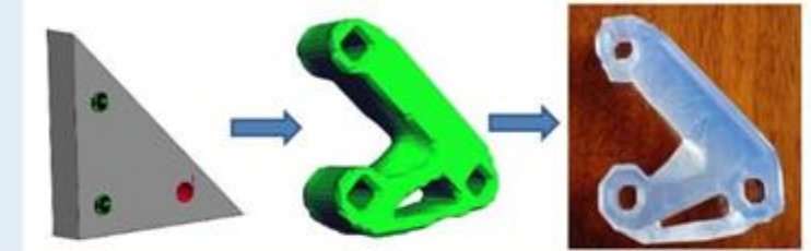
Figure 1: Topology optimization can create a light weight part for 3D printing.
